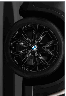
Star Spoke High-gloss Black light alloy wheels (Style 491) 20 x 10.0 front; 20 x 11.0 rear; and 275/40 front; 315/35 rear run-flat performance tires 1,2,3
