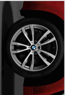
Double Spoke light alloy wheels (Style 469M) 20 x 10.0 front; 20 x 11.0 rear; and 275/40 front; 315/35 rear run-flat performance tires 1,2,3
